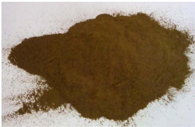
Figure 2.1: sewage sludge ash
