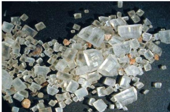
Figure 2.4: Struvite crystals from the Airprex process (STOWA, 2012)
