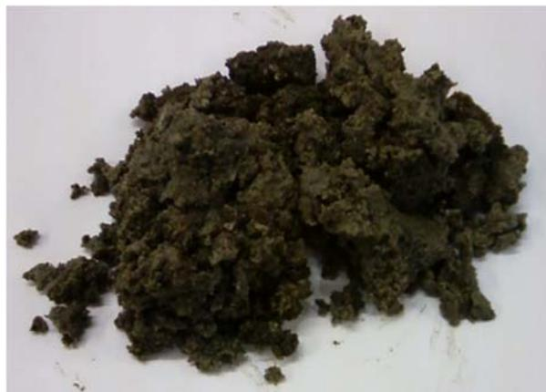
Figure 2.5: struvite from the Anphos process as received in bulk
