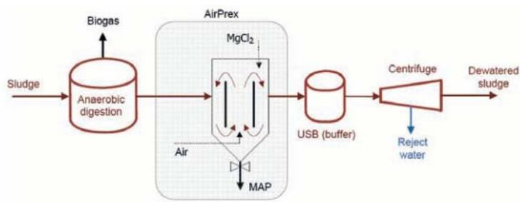
Figure 2.3: schematic of the Airprex process' position in a WWTP (STOWA, 2012)
